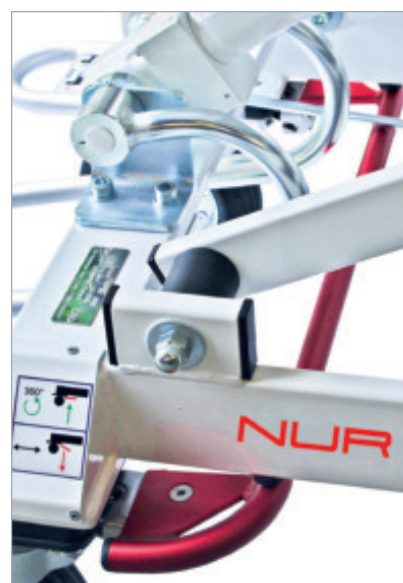
Direction lock also as retrofit kit 2018 NRS-R for RTH Stretcher transporter 2018
