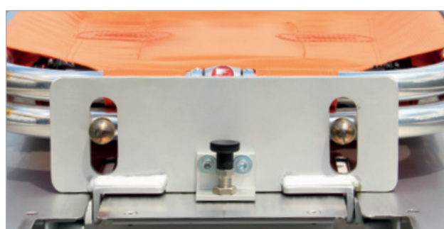
Stretcher 12-2 secured with the mounting plate
