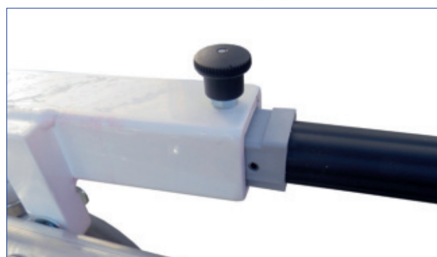
Safety locks prevent telescopic handles from slipping out when chair is folded
