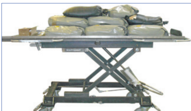
Static load test on the prototype
