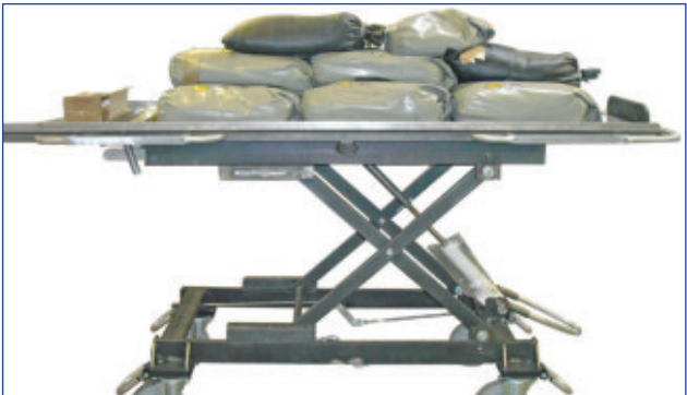
Static load test on the prototype
