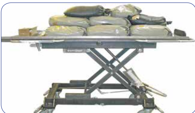
Static load test on the prototype
